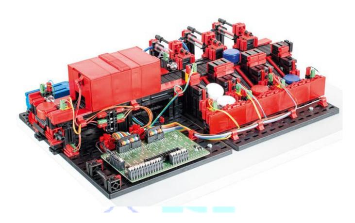
Detects workpieces of different colors and sorts them via a conveyor belt into the provided storage unit.
