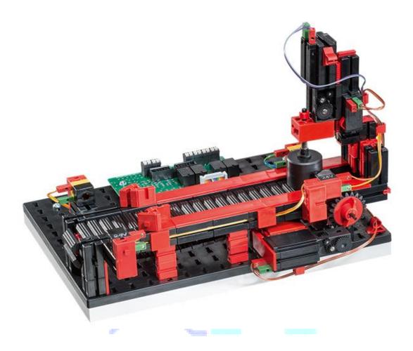
The punching machine with conveyor belt simulates conveying and punching of workpieces. The model is ideally combinable with the training model "3-axis robot with gripper".
